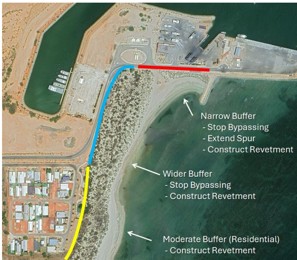
Figure 6-29: Segments for Neale Cove Erosion Management
