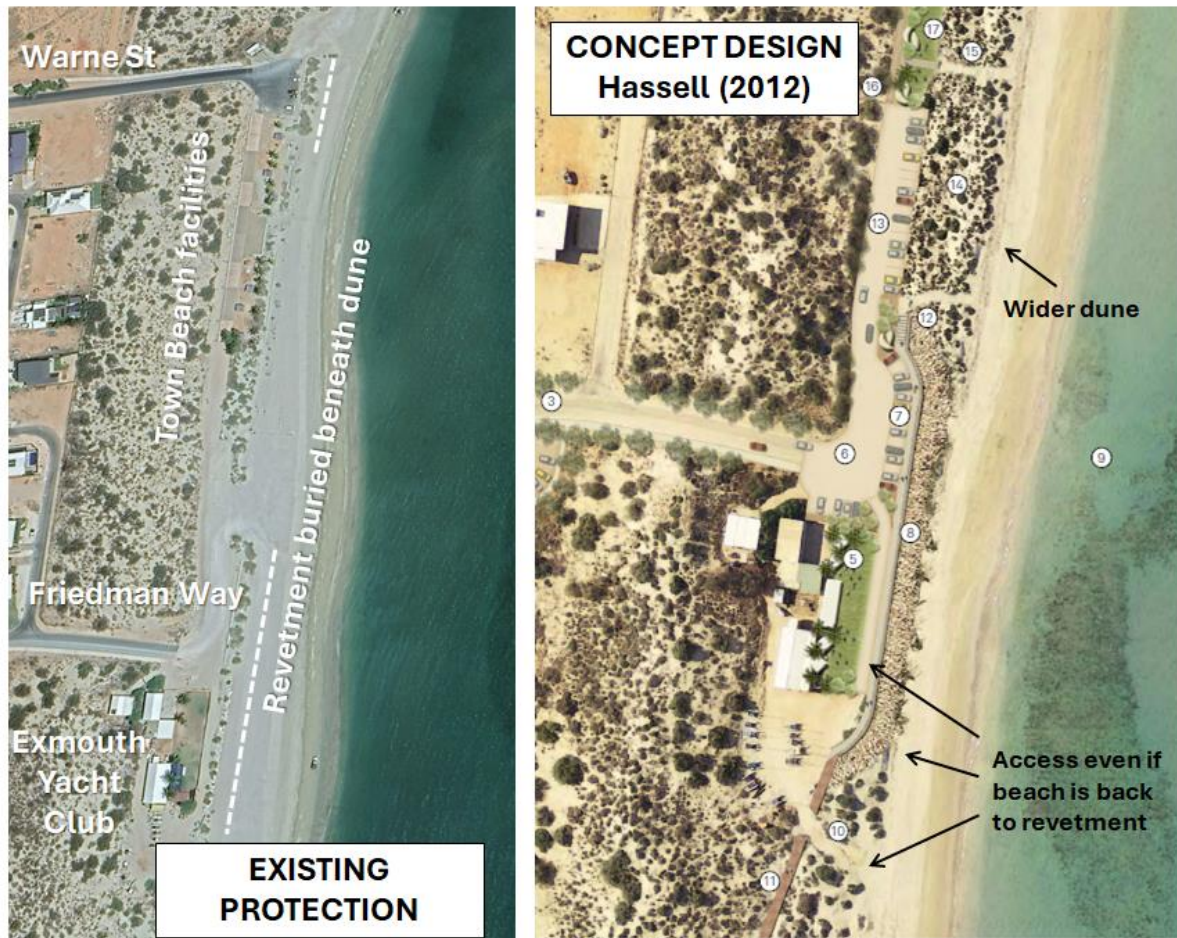
Figure 6-11: Existing Protective works and 2012 Concept Design for Yacht Club site Note that dune loss has affected the original design intent
