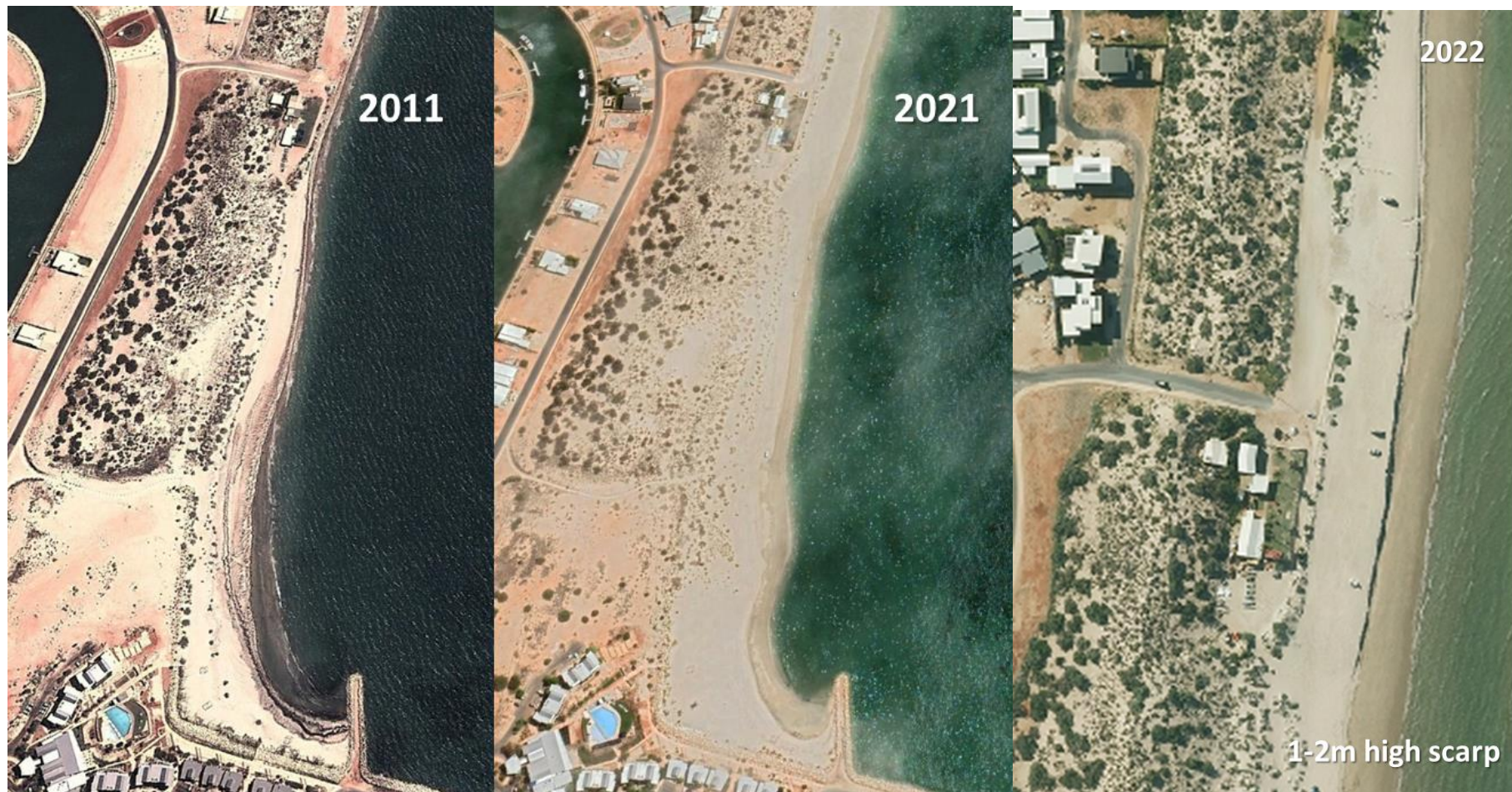
Figure 6-7: Beach utility and access on Town Beach 2011 – scarping due to transport reversal; 2021 – Subsequent progressive accretion; 2022 – scarping due to sand placement
