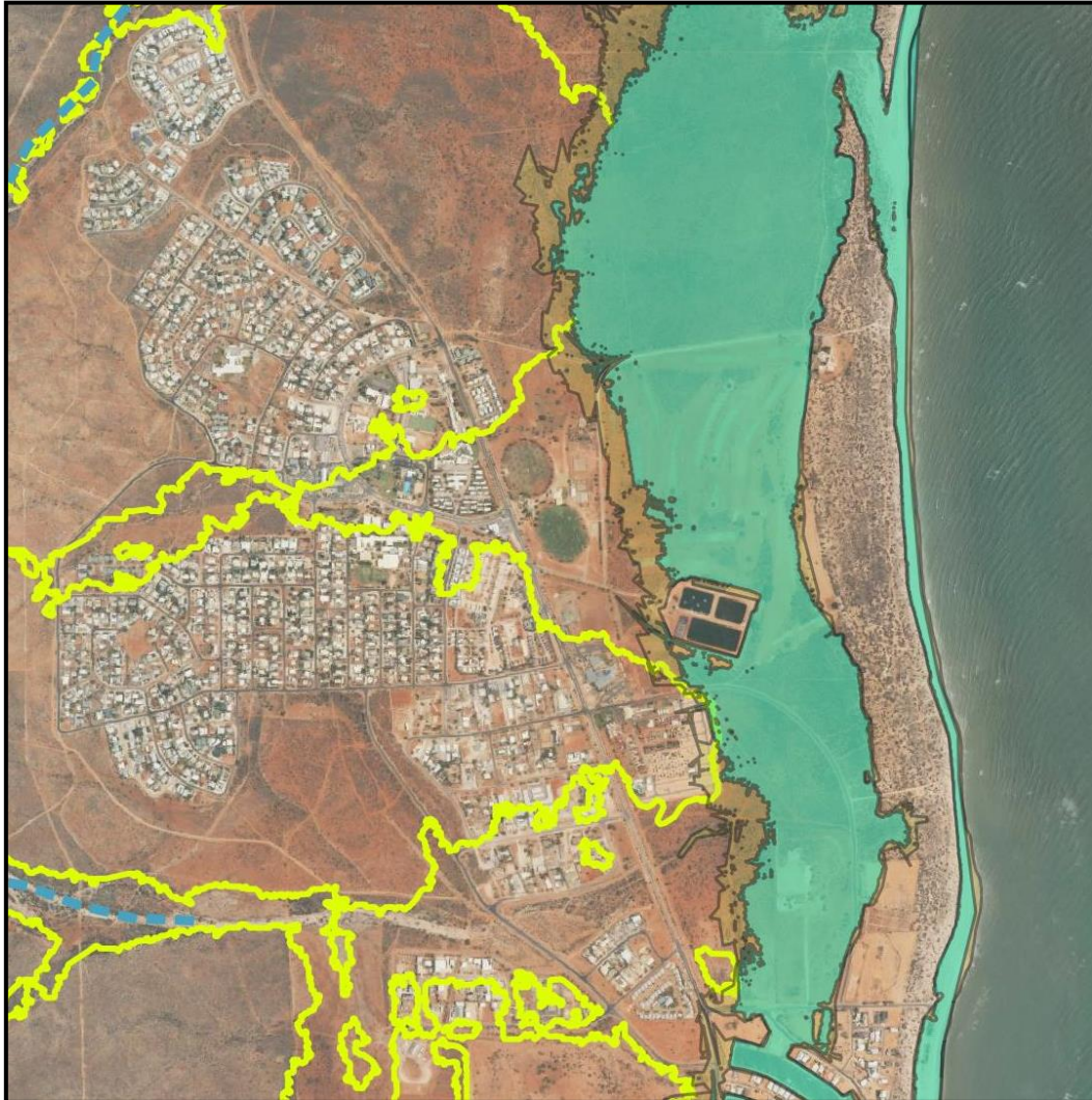
Comparison of Floodplain Areas subject to Runoff Flooding (yellow) and potentially subject to Coastal Inundation (green) with inclusion of +0.9m sea level rise.
