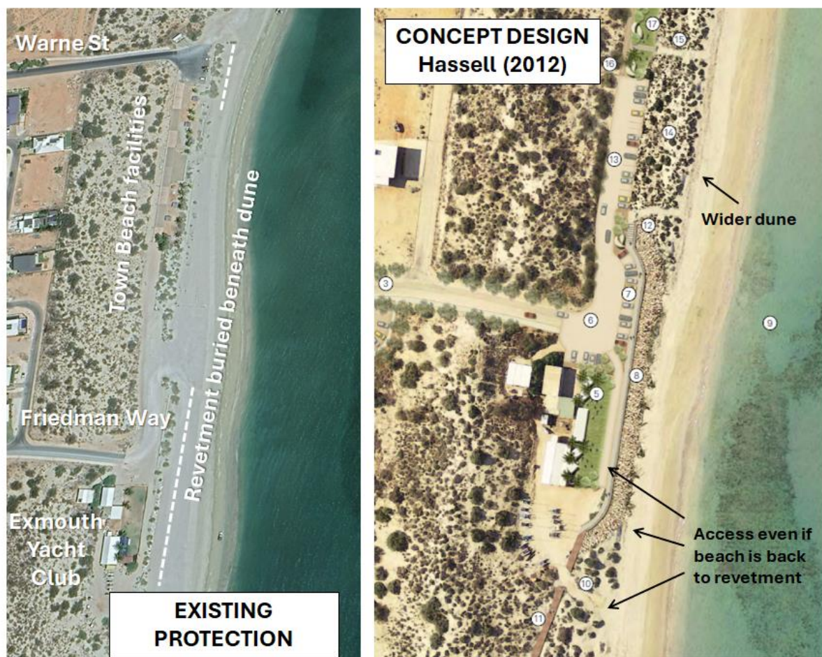
Figure 6-11: Existing Protective works and 2012 Concept Design for Yacht Club site Note that dune loss has affected the original design intent
