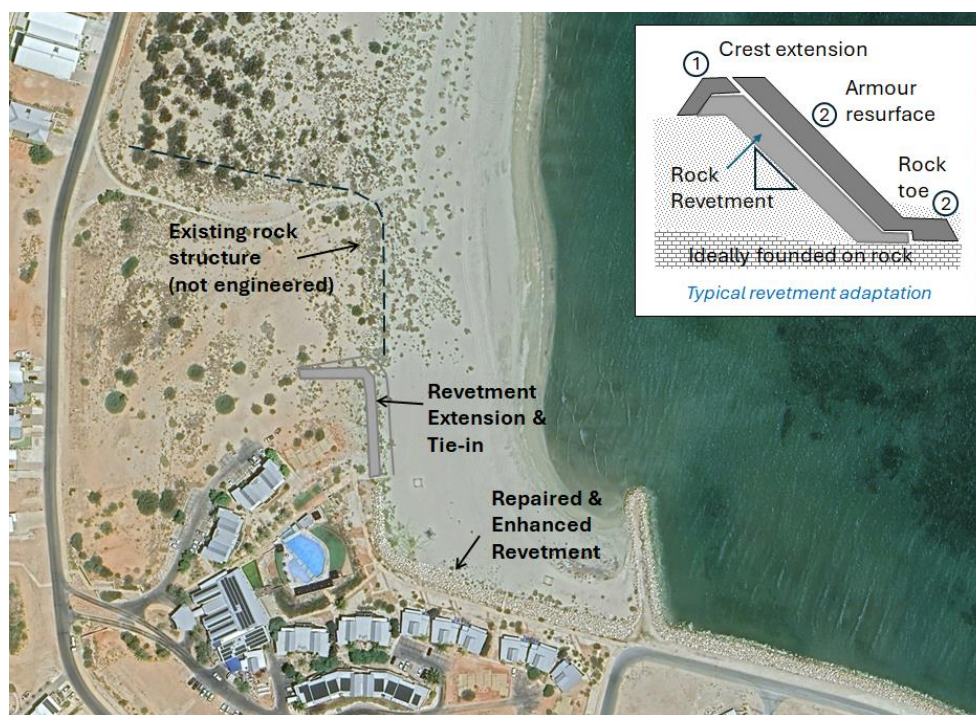
Figure 6-21: Local revetment extension and adaptation adjacent to Mantarays
