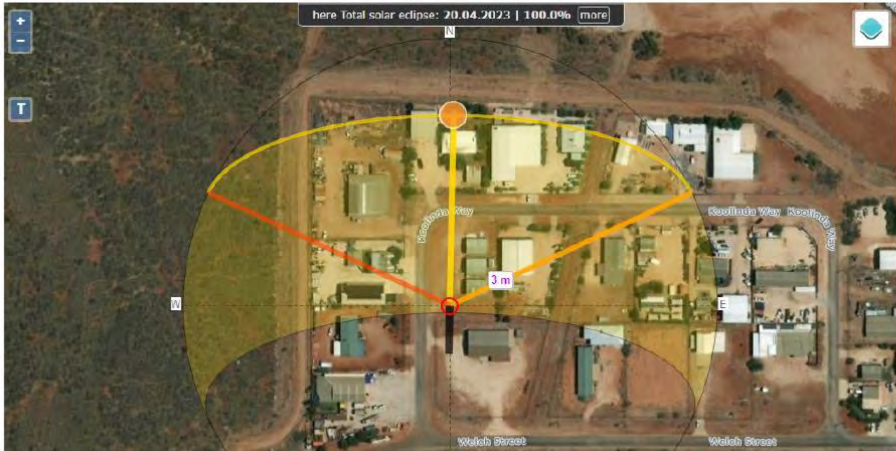
Extent of shadowing for tower on shortest day of year (21 June 2022) at 12:22am. Note that width of actual shadow will be smaller than shown on image Source: SunCal, 2022
