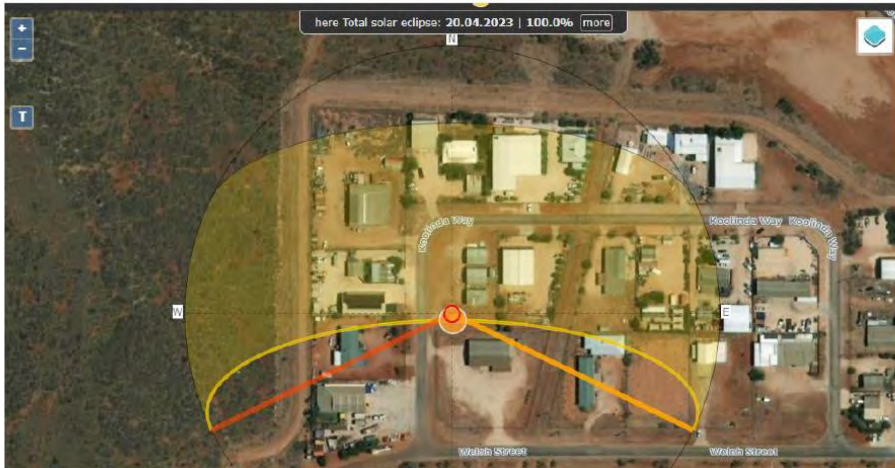
Extent of shadowing for tower on longest day of year (22 December 2022) at 12:22pm. Note that width of actual shadow will be far slimmer than shown on image Source: SunCal, 2022
