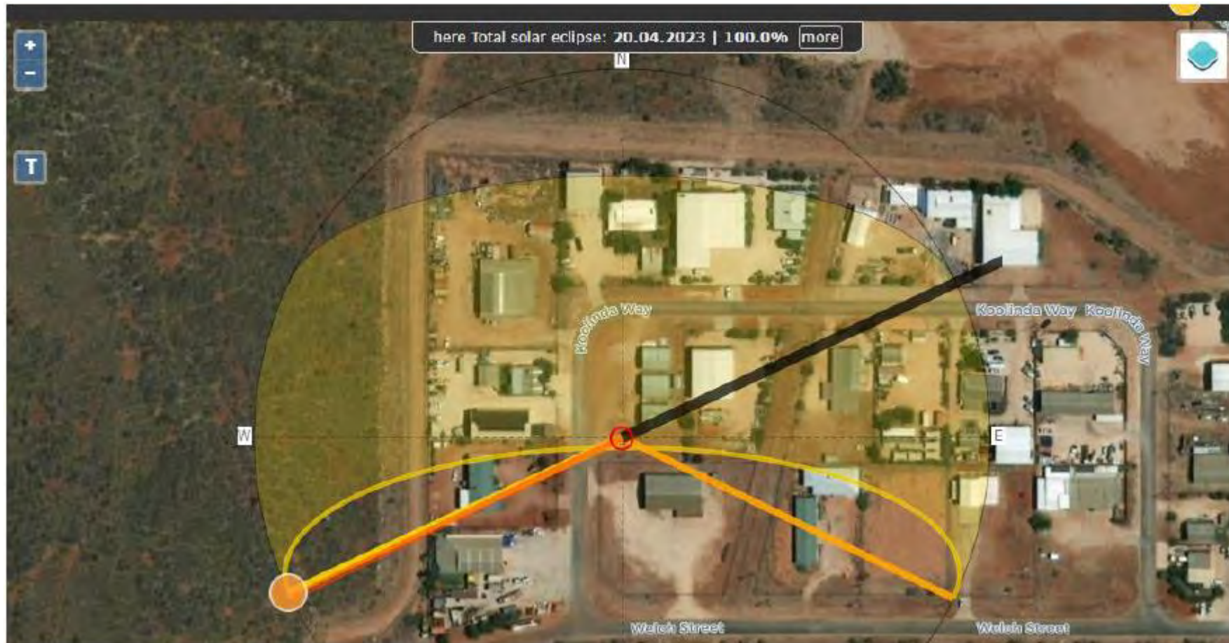
Extent of shadowing for tower on longest day of year (22 December 2022) at 7:02pm. Note that width of actual shadow will be smaller than shown on image Source: SunCal, 2022
