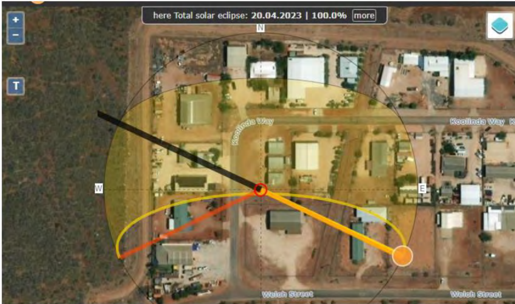
Extent of shadowing for tower on longest day of year (22 December 2022) at 5:40am. Note that width of actual shadow will be far slimmer than shown on image Source: SunCal, 2022
