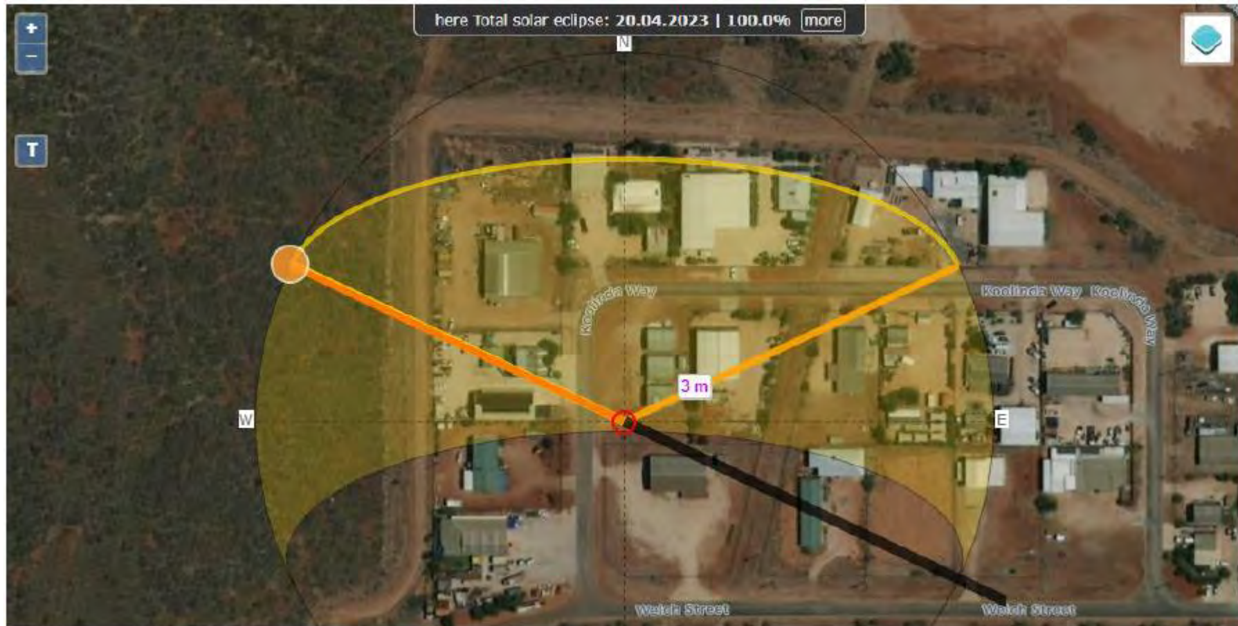
Extent of shadowing for tower on shortest day of year (21 June 2022) at 5:47pm. Note that width of actual shadow will be smaller than shown on image Source: SunCal, 2022
