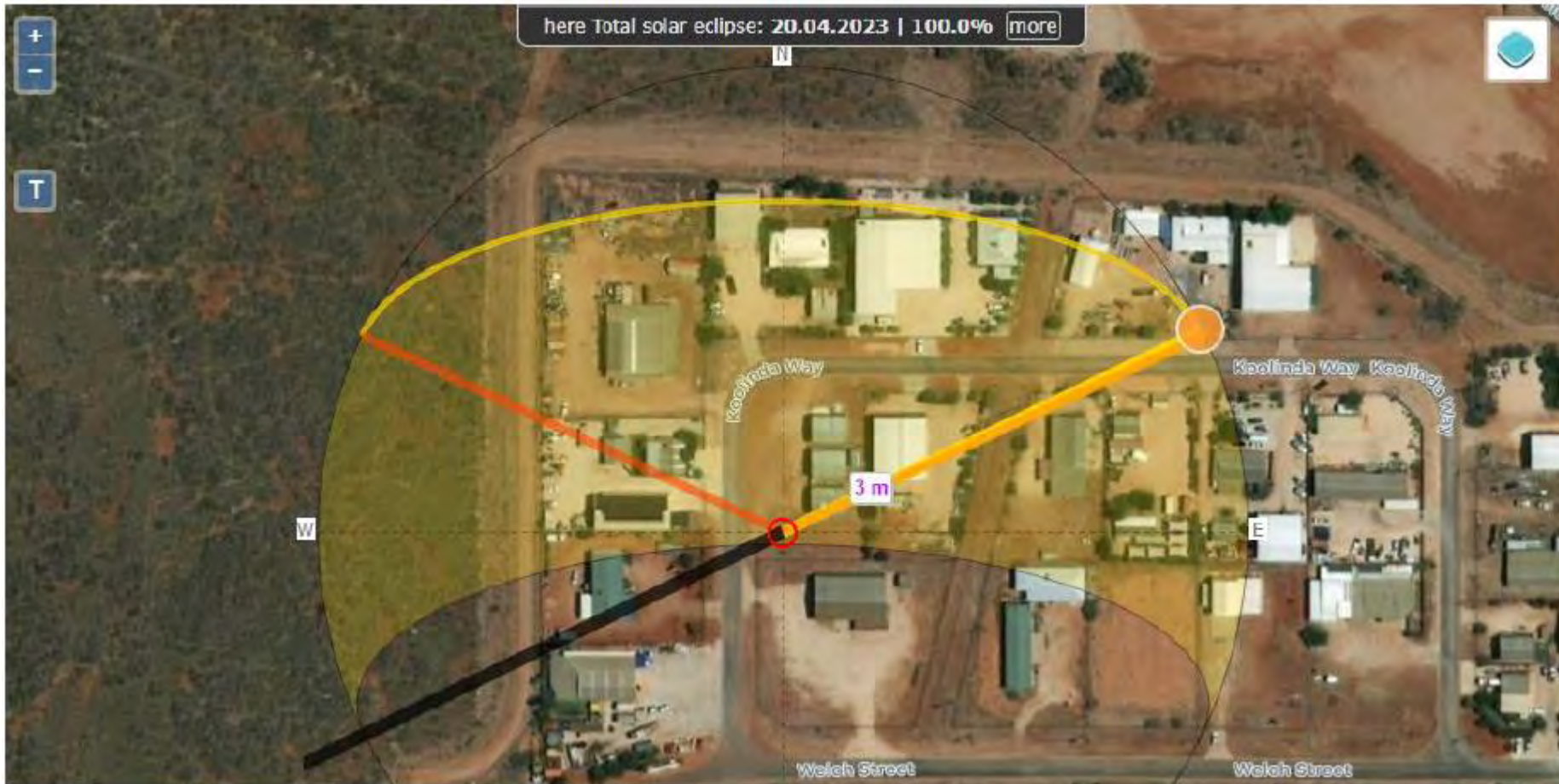
Extent of shadowing for tower on shortest day of year (21 June 2022) at 7:09am. Note that width of actual shadow will be smaller than shown on image Source: SunCal, 2022
