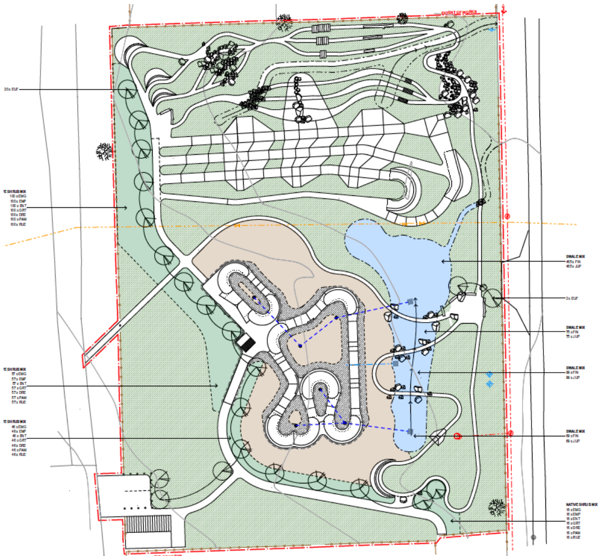
Figure 1: Design of the Exmouth Bike Park to be undertaken in separable portions and/or stages (with separate Pump Track, Jump Lines and Skills Loop)
