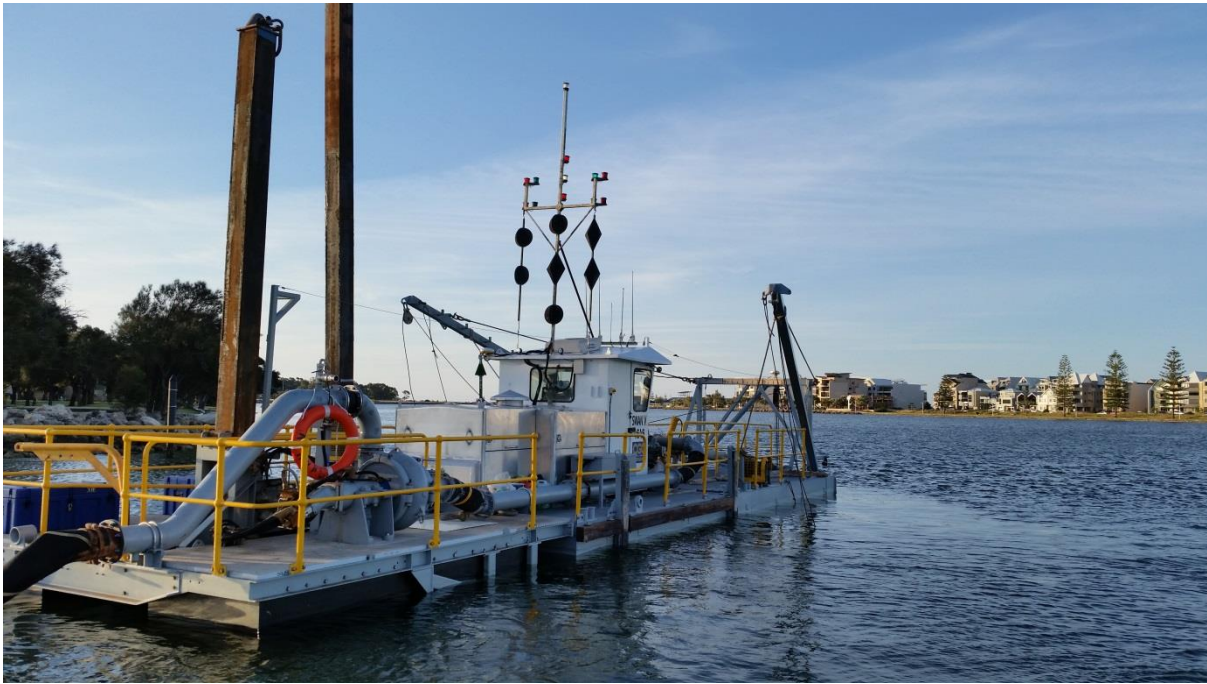
Photo 1: Typical Bucket Wheel Dredger
